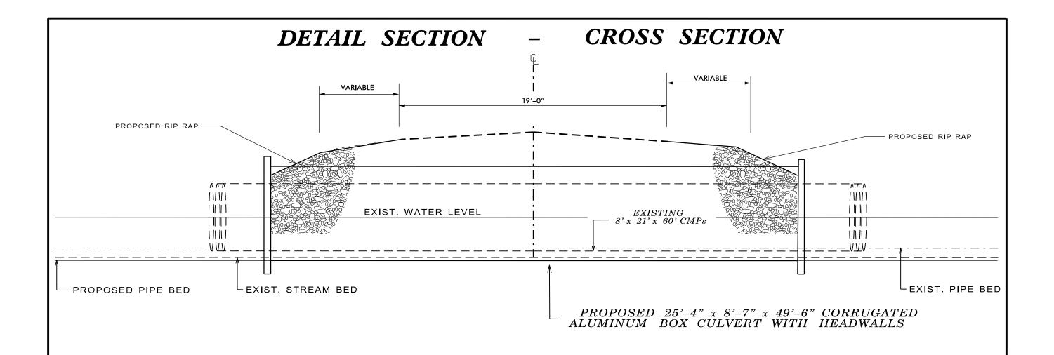
NOTES: \* PROPOSED 25'-4" X 8'-7" X 49'-6" CORRUGATED ALUMINUM BOX CULVERT TO BE BURIED 1.0' BELOW EXISTING STREAM BED
